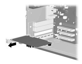
removing an expansion card on the \$0000/8000 (\$0000 shown)
